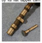
Zinc is an anti-wear additive and an absolute necessity for older flat tappet engines. However in new modern engines, zinc has been found to damage the catalytic converter and together with auto manufacturers, oil producers have reduced the level of zinc formulations in oils labeled "SM".
